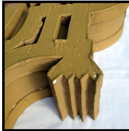
Attention to detail. Built up by layering pine lumber.
